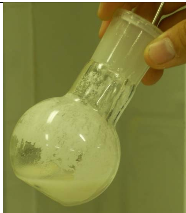
Session 1: the product after crystallization (addition of methanol and then diethyl ether)
