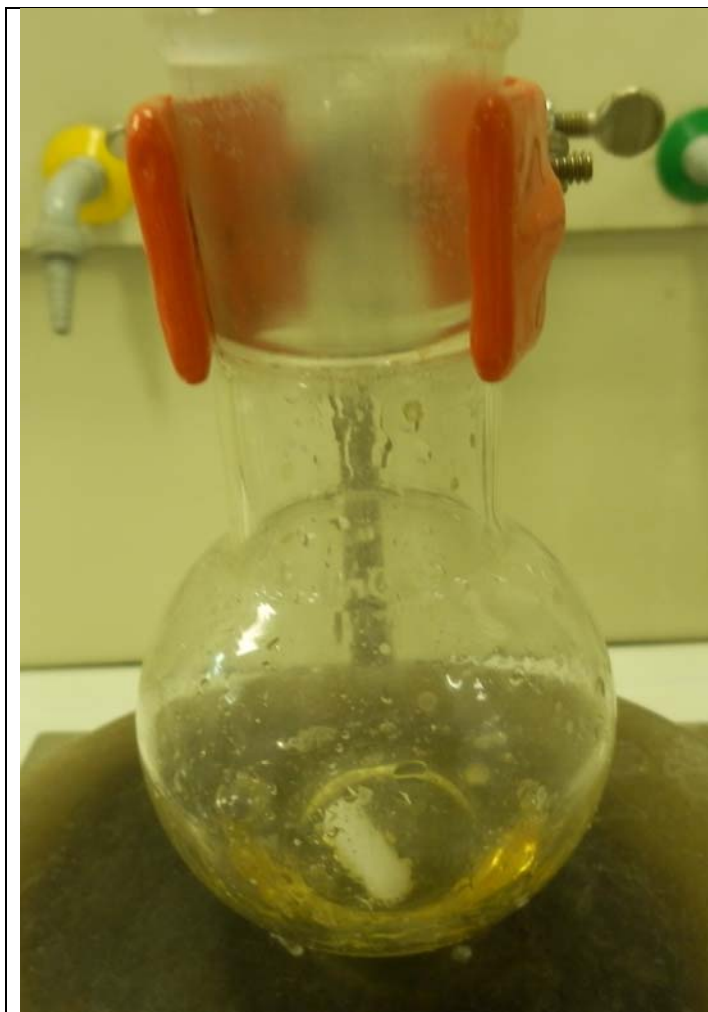
Session 1: the flask containing crude product after methanol distillation
