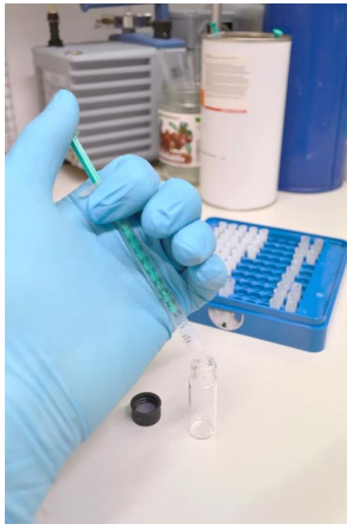
Scheme SM 18.3.10 Samples taken from the reaction are filtered with a syringe filter.
