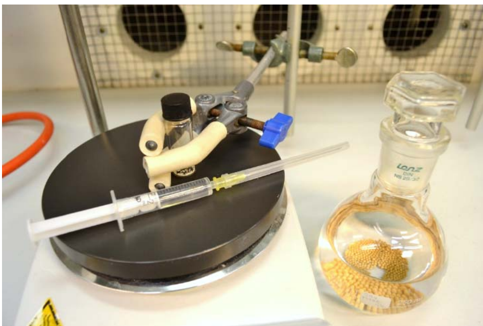
Scheme SM 18.3.8 Addition of 1.7 mL dry MTBE (4 Å mol. sieves) using a plastic syringe.
